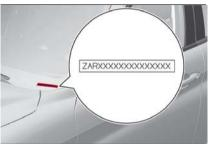
1001650001EM Vehicle Identification Number This number is also printed on the chassis at the front left shock absorber and can be seen by opening the engine compartment hood.
