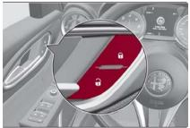
Door Lock And Unlock Switch Panel
