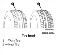
These indicators are molded into the bottom of the tread grooves. They will appear as bands when the tread depth becomes a 1/16 of an inch (1.6 mm). When the tread is worn to the tread wear indicators, the tire should be replaced. Refer to "Replacement Tires" in this section for further information.
