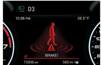
The system may lightly brake to warn the driver if a potential front end collision is detected (limited braking). Signals and limited braking are intended to allow the driver time to intervene.
