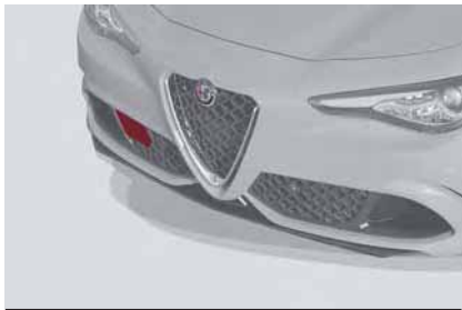
Front Bumper Radar Location
