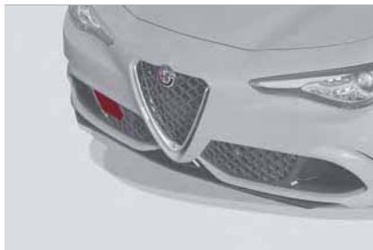
Front Bumper Radar Location
