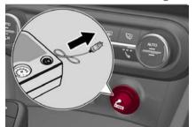
Inserting Plug Into Outlet
